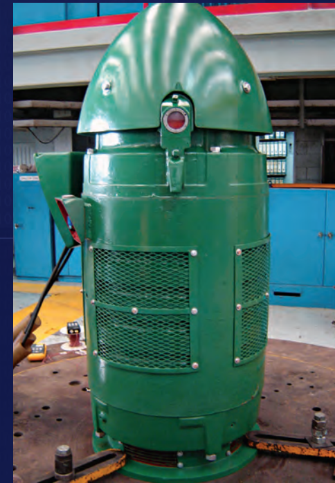
Obsolete Westinghouse 509P frame with brand new internal components, custom designed to extend motor life.
